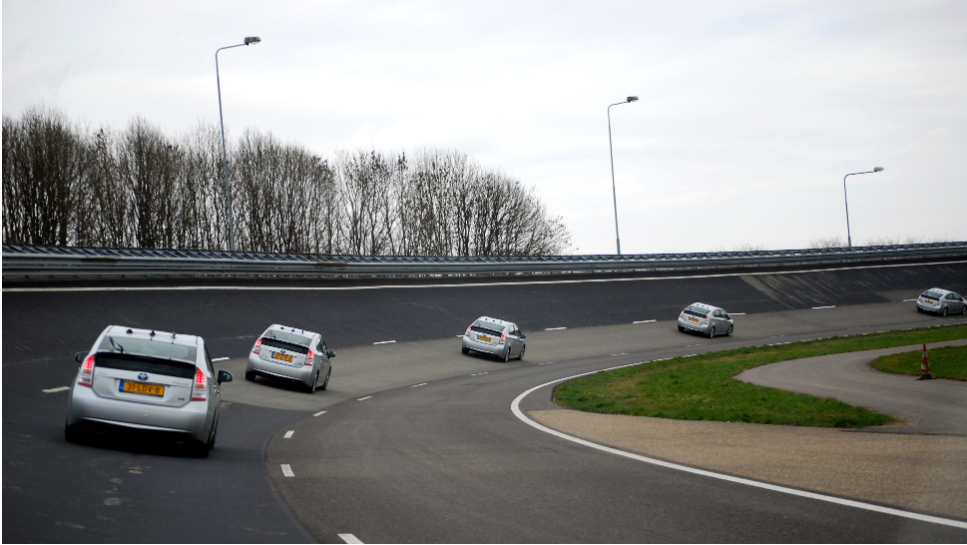
Figure 2.2: Prototype testing of a CACC system during the Connect & Drive project. Picture taken by Bart Klaassen.
